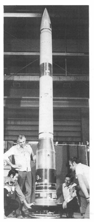
ROCKET PAYLOAD, 16.5 ft. in length and weighing 550 lbs., is checked for spin balance in the Mass Properties Lab in Bldg. 892 by Ted Krein (1525), standing, project leader; Ernie Niper (1525); Hovey Corbin (1525), and Harry Blechinger (1137). Two of the payloads will be launched into the shadow of a total eclipse off the coast of East Africa Feb. 16.
